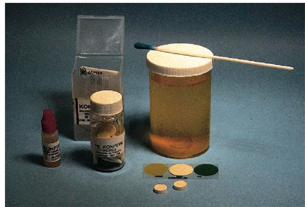
ONPG and MUG are enzyme substrates bound to specific indicators. When the enzyme galactosidase hydrolyses the colorless ONPG (O-nitrophenyl-β-D-galactopyranoside), it produces galactopyranose and O-nitrophenyl, which is yellow (figure 47.4a).
