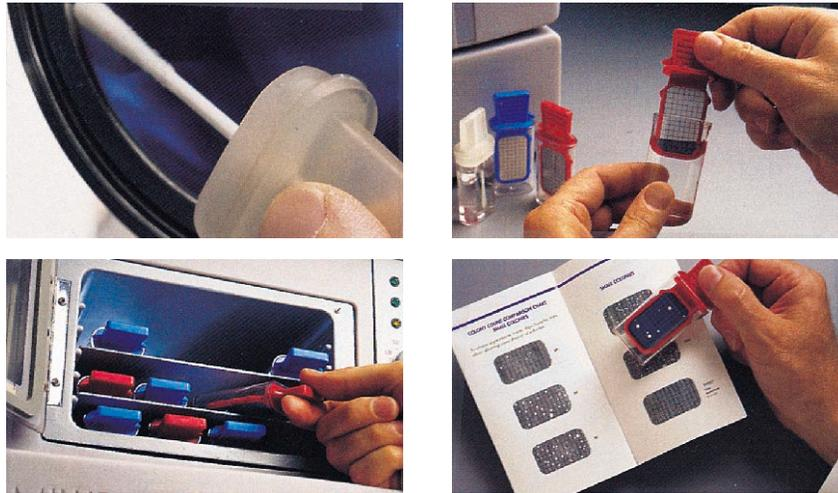
**Figure 44.3 Small and Large Colony Counts.** Simply align the sampler with photo showing same density of colonies and record that number.
